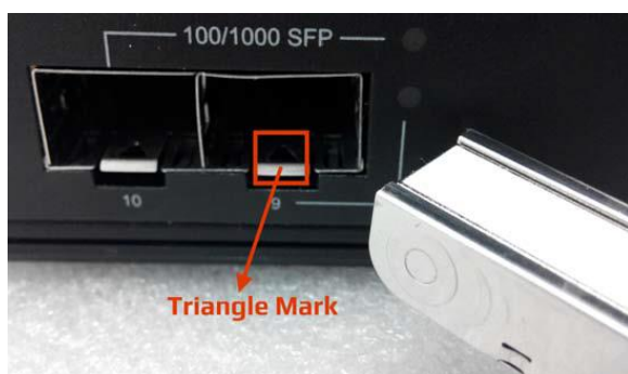
Figure 2.6 - Transceiver to the SFP Slot
