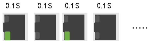
Figure 2.6 - PoE Over Current LED Sequence
