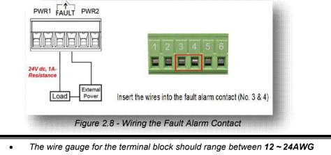
If only using one power source, jumper Pin 1 to Pin 5 and Pin 2 to Pin 6 to eliminate power fault alarm.
