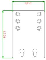
Figure 3.5 Wall Mounting Bracket Dimensions
