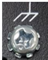
Figure 2.15 - Grounding screw symbol
