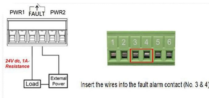
Figure 2.8 - Wiring the Fault Alarm Contact
