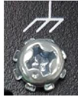
Figure 2.15 - Grounding screw
