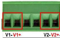
Figure 2.6 - Power Terminal Block
