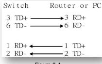
Figure 2.4 Straight-Through Cable Schematic
