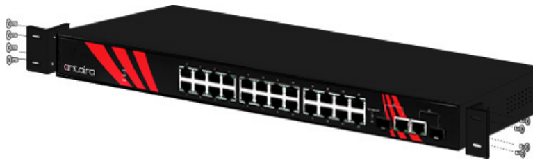
Figure 3.1 - Attach Mounting Plates with Screws
