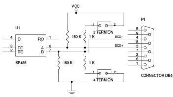
The image above shows how the TERM ON pins modifies the circuit The TERM ON pins can apply 1K pull-up & pull-down resistors
