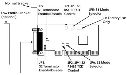
J2: DB25M Connector, to DB25F-to-DB9MX2 Octopus Cable
