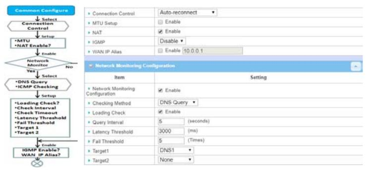
There are some important parameters to be setup no matter which Ethernet WAN type is selected. You should follow up the rule to configure.
